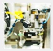
The IEC 63171-6 compliant T1 Single Pair Ethernet connector is the first choice for industrial applications by the international standards committees ISO/IEC, TIA and IEEE. Based on a modular system, applications from IP20 to IP65/67 are possible. The Mini PushPull brings the T1 SPE mating face from the field to the machine and enables quick, easy and reliable installation.
